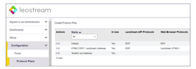
Each protocol plan defines the display protocol used when the user logs in using different client types, such as Leostream Connect and thin clients, the Leostream Web client, and PCoIP clients. You configure the display protocol for each of these client types separately, using the appropriate section in the protocol plan.
