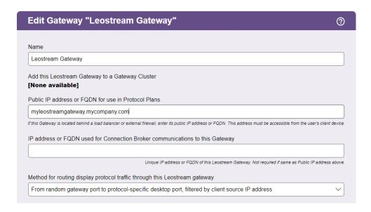
If you are required to use the protocol-specific port 443 for the RAP – VDI traffic and you use your Leostream Gateways to forward Connection Broker login traffic, you must configure your Leostream Gateway to use a port other than 443. For instructions on changing the default Leostream Gateway port, see the **Leostream Gateway Guide**.
