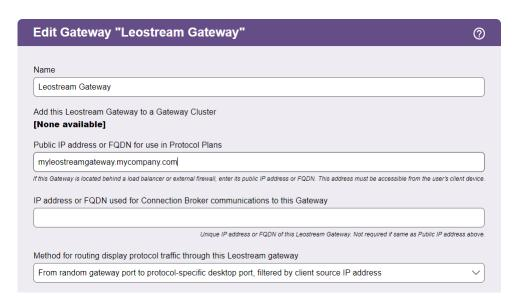
If you are required to use the protocol-specific port 443 for the Scyld Cloud Workstation traffic and you use your Leostream Gateways to forward Connection Broker login traffic, you must configure your Leostream Gateway to use a port other than 443. For instructions on changing the default Leostream Gateway port, see the **Leostream Gateway Guide**.
